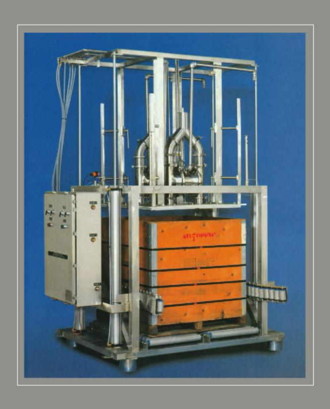
The Murzan TUS-50 is the ideal solution for emptying 1000 litre (IBC) Intermediate Bulk Containers and standard 1135 litre (300 US gallon) wooden totes of highly viscous products. Used in applications that no pump alone can handle, the Murzan TUS-50 unloads viscous pastes and concentrates cleanly and quickly. Additionally, the Murzan TUS-50 conforms to FDA requirements for approved materials, is CIP capable, and incorporates the USDA listed Murzan PI50.
